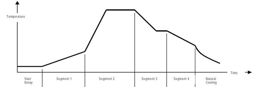
In the above example program segments 1 to 4 are used. Segments 5-9 are spare. Natural cooling occurs after execution of the final program segment. Dwell (soak) times for segments 1 & 4 are shown set to 00:00.
