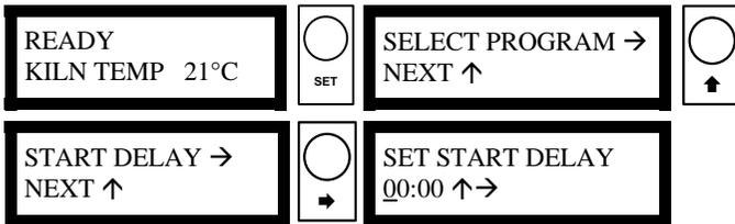
Choose the **START DELAY** item on the menu with the **→** key. Set the required delay in the range 00:00 to 99:59 (hours:mins) with the **↑** & **→** keys. Select this with the **→** key.
