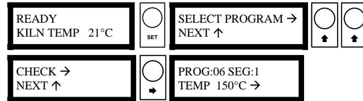
The **→** key is now used to step through each segment of each program in the order in which they will be executed as shown in this example:-
