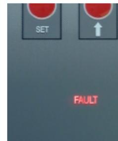
If the optional over-temperature trip module is installed a red FAULT lamp illuminates when an over-temperature error condition occurs. The trip turns off heating power. Turn off mains power to the kiln & controller & investigate the cause of the error. The trip is automatically reset by removal of the mains supply to the controller. If the fault is still present the trip will operate again about 5 seconds after re-powering the controller.
