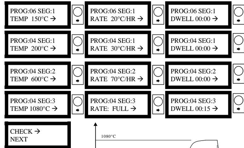
In the above example programs 6 & 4 are linked together. The ramp rate for segment 3 is shown as **FULL** because this has been set to 999°C/hour.
