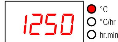
**➡** then displays the soak temperature in the range 0 to 1320°C. This can be altered with the **⬆** & **⬇** keys. The SOAK TEMPERATURE lamp on the mimic display will flash.
