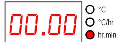
The next push of the **➡** key displays the start delay time in the range 00.00 to 99.59 (99 hours 59 mins). This can be altered with the **⬆** & **⬇** keys. The DELAYED START lamp on the mimic display will flash.
