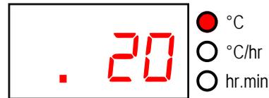
If the left-hand decimal point is on then the keyboard is locked & the ST316 will not respond to the START/STOP key. Press the  $\uparrow$  &  $\downarrow$  keys together & hold down for 5 seconds to unlock.
