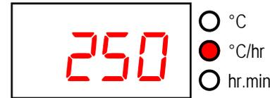
**➡** then displays ramp rate 2 in the range 1 to 399°C/hr or *FULL* or *End*. This can be altered with the **⬆** & **⬇** keys. The RAMP 2 lamp on the mimic display will flash.
