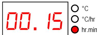
The next push of the **➡** key displays the soak time in the range 00.00 to 99.59 (99 hours 59 mins). This can be altered with the **⬆** & **⬇** keys. The SOAK TIME lamp on the mimic display will flash.
