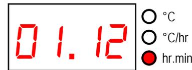
If a delayed start has been set then pressing the START/STOP key causes a time delay to start. The time remaining is shown on the display—this counts down once per minute. The DELAYED START lamp on the mimic panel will light. The centre decimal point will flash once per second.
