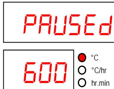
As a warning during pause a double beep is sounded every 10 seconds, the display scrolls *PAUSED* for 5 seconds then shows the kiln temperature for 5 seconds.
