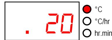
If the left-hand decimal point is on then the keyboard is locked & the ST315 will not respond to the START/STOP key. Press the  $\uparrow$  &  $\downarrow$  keys together & hold down for 5 seconds to unlock.
