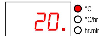
If no delayed start has been set (00.00) then pressing the START/STOP key causes firing to commence immediately. Either the Heating or Cooling lamp on the mimic panel will light. If kiln heating is required then the right-hand decimal point on the display will light while heating power is being applied to the kiln.
