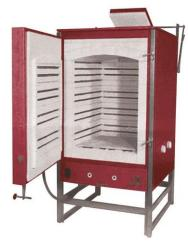
The Firebird 'K' range of front-loading kilns is an 8 model range covering the size range 106 to 708L (3.75 to 25 cubic feet). Elements are inserted into the side walls, back wall, base & door. A roof damper fitted to models of size 283L (10 cubic feet) and above.
